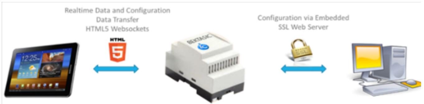
For typical usage only port 3800 is needed to be accessible from Internet for client applications. Configuration port is not recommended to open to Internet for enhanced security.
